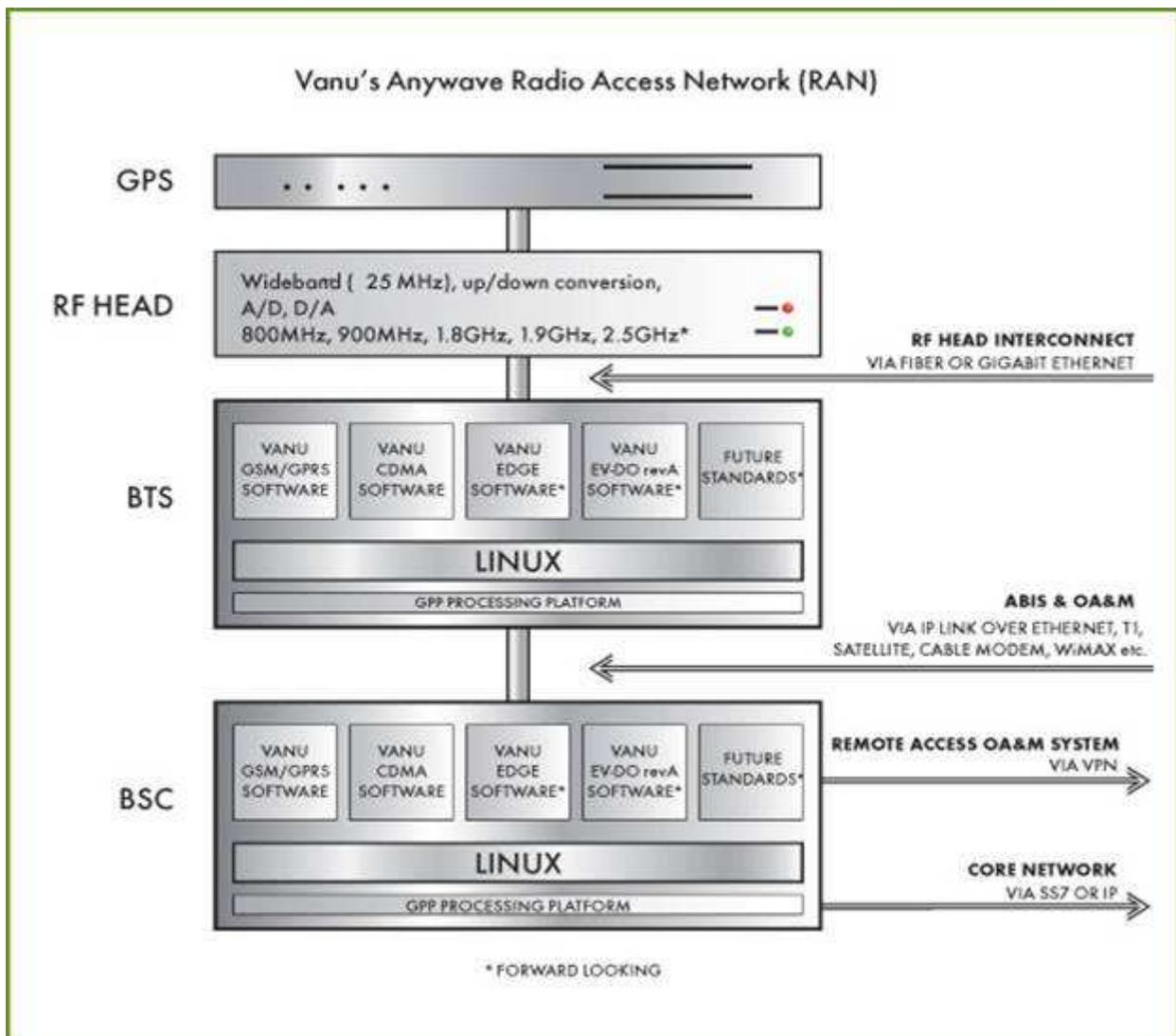
The Anywave Base Station is part of the Anywave RAN, which uses native IP throughout for signaling, voice, data, and management. Any desired backhaul links can be used (e.g. T1/E1, Ethernet, satellite and microwave). Because IP is used throughout the Anywave RAN, cost-effective commercial switches, bridges and routers are available, as well as tools for network monitoring and maintenance. The burst-like data traffic characteristic of 2.5G and 3G
