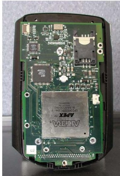
Figure 4: Interface card with iPAQ sleeve for scale.
